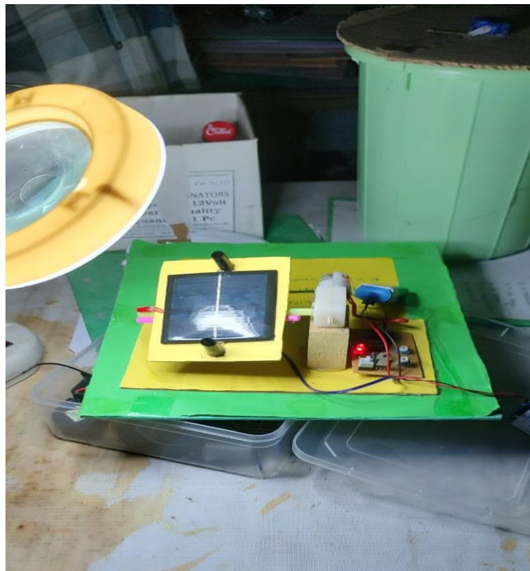
SOLAR TRACKER EQUIPMENT
